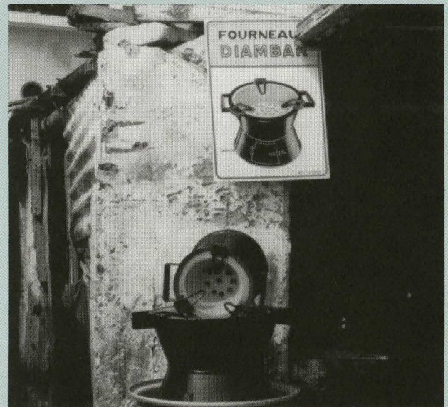
The Diambar stove features an increased height, curved handle and other improvements requested by women users.
