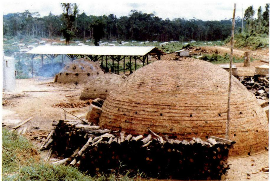
*The first firing of the 5 m brick kiln nears completion.*
