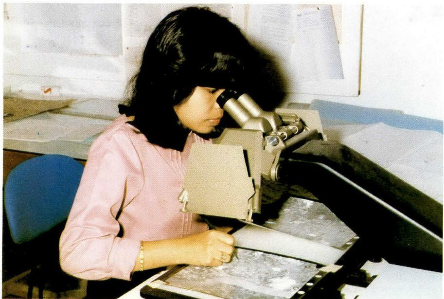
*Production of maps from aerial photography by using a stereoscope.*
