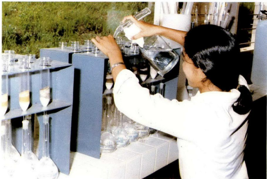
*Filtration of liquid soil samples.*
