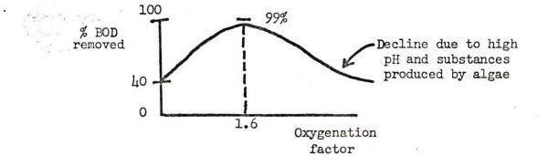
Because the optimum oxygenation factor  $\simeq$  BOD/O2 conversion, one may substitute BOD for C  $_{\rm c}$
