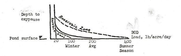
When the oxypause reaches the surface, the whole pond becomes anaerobic.
