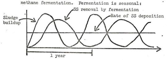
Therefore sludge must be balanced over the year. There will always be some build-up due to grit (1-10 ft<sup>3</sup>/mg; usually 1-3 ft<sup>3</sup>/mg) and to residuals from sludge (0.1 ft<sup>3</sup>/cap/year).
