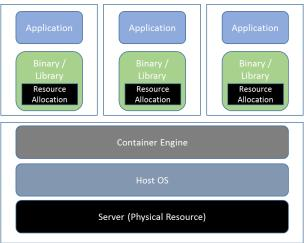
Unlike traditional virtual machines, containers do not have a guest operating system installed, but it does require that the physical server have a host operating system. The container itself contains the application in addition to all the components needed for that application and uses the host operating system. This means there is less wasted computing making for a more efficient system, and is also easier to move when needed.
