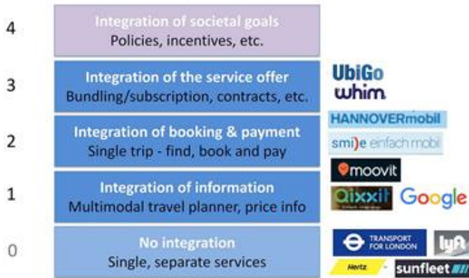
MaaS topological scheme, including MaaS levels and examples of these (Sochor et al., 2018)
