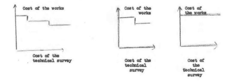
The gaps correspond to the discovery of phenomena (a strip of rocky ground, for ememple) that can easily be avoided by modifying the layout of the road. Such phenomena, had they not been discovered, would have resulted in an increase in the cost of the works.
