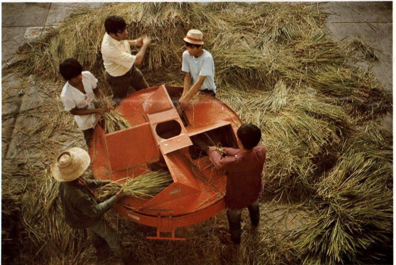
Dr. Amir Khan, an American citizen, works on a new table thresher with a capacity of 250-350 kg per hour.
