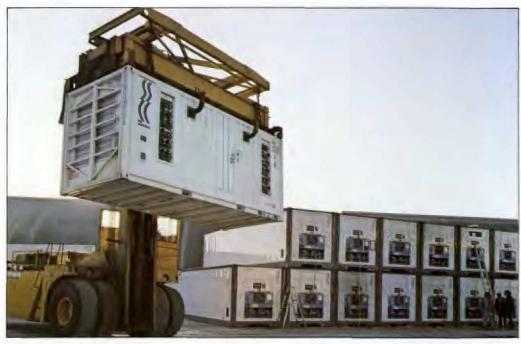
Moving a Power Pack to recently discharged 40ft refrigerated containers.
