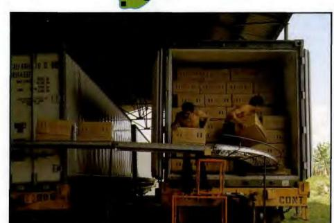
Left: Bananas being packed into railmounted 40ft refrigerated containers at the plantation. The fruit is constantly ventilated and maintained at a precisely controlled temperature through rail, sea and road transit, and is not handled until it reaches the ripening warehouse at the eventual destination. This reduces wastage and improves quality, allowing premium retail prices to be obtained.
