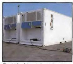
Two 20ft refrigerated containers in a transit depot. The diesel engines fit within the ISO perimeter.
