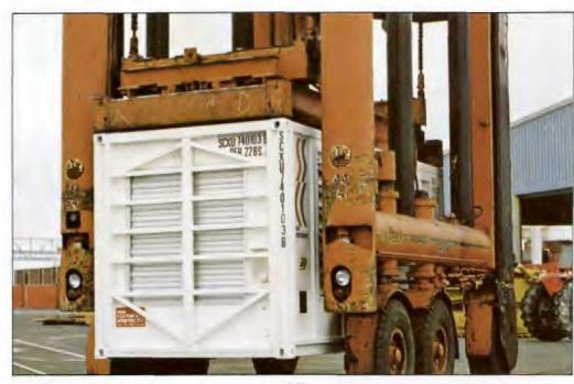
The Power Pack being moved by a straddle carrier.
