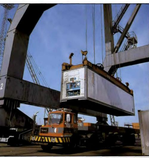
Above: A 40ft Carrier reefer, with a cargo capacity of 1956 cu ft (55.39 cu m) being loaded on to a container chassis for onward delivery by road.
