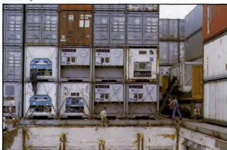
Right: A Sea Containers' Power Pack being connected to reefers on board ship.
