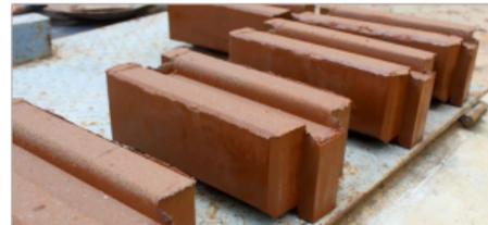
Material: laterite, cement, and coarse sand
