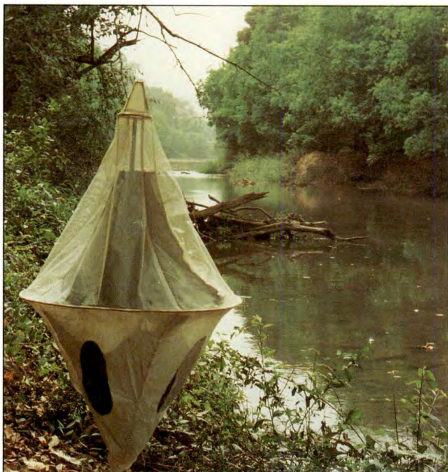
A conical trap, one of several different types of traps developed to catch tsetse flies.
