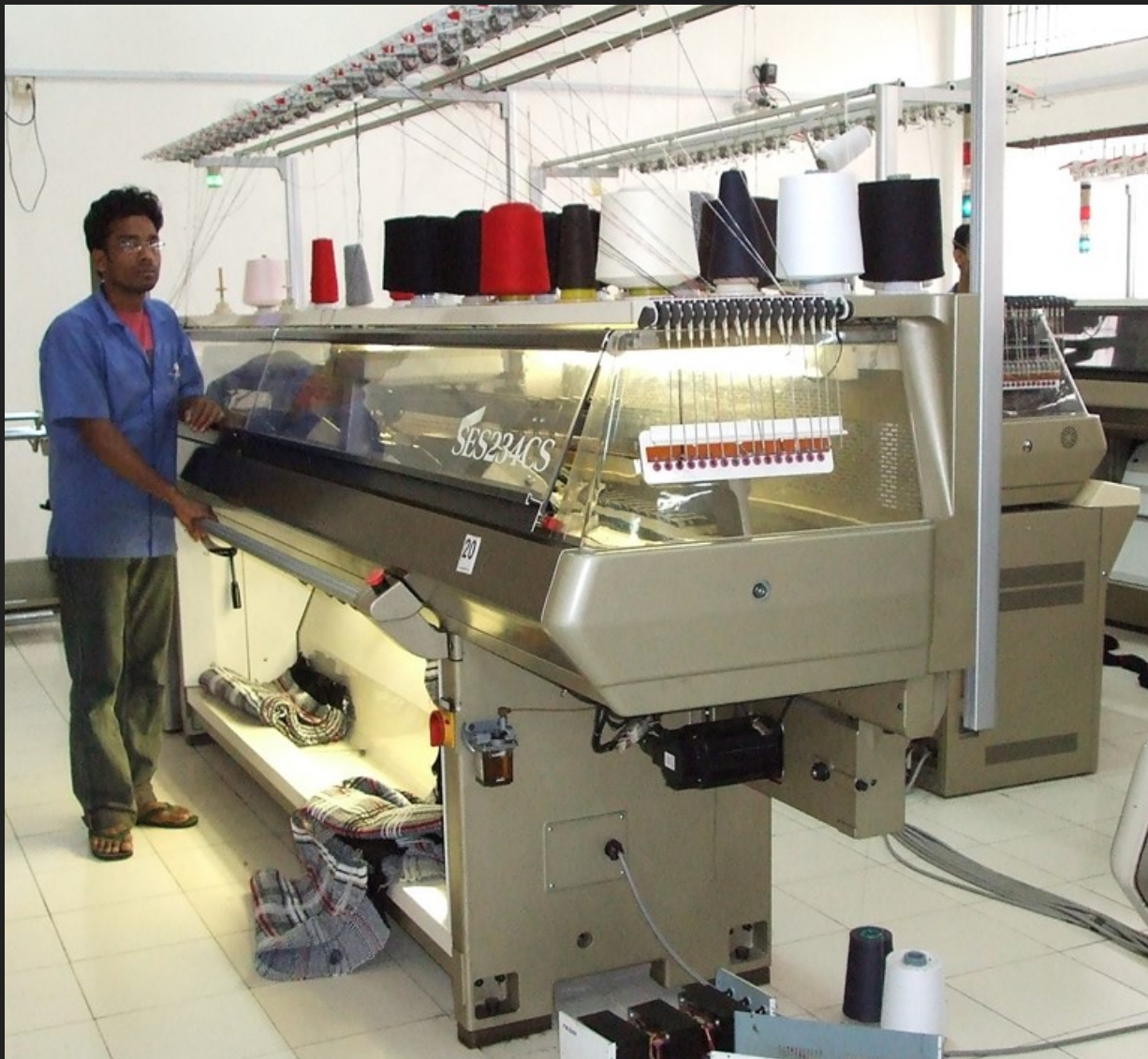
Shima Seiki Mfg, Ltd. invented the Wholegarment Knitting Machine in 1995. The above is another model of flat knitting machine made by Shima Seiki. (Bangladesh, 2008)
