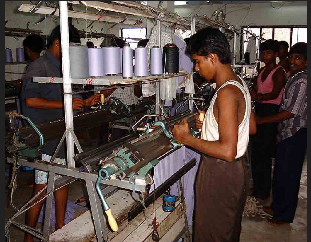
A manually operated flat knitting machine (Bangladesh, 2001)
