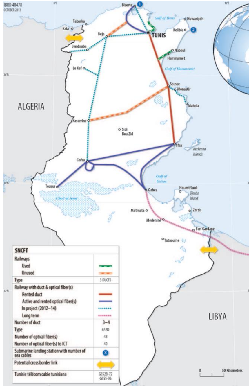
Figure 35: SNCFT fiber optic network
