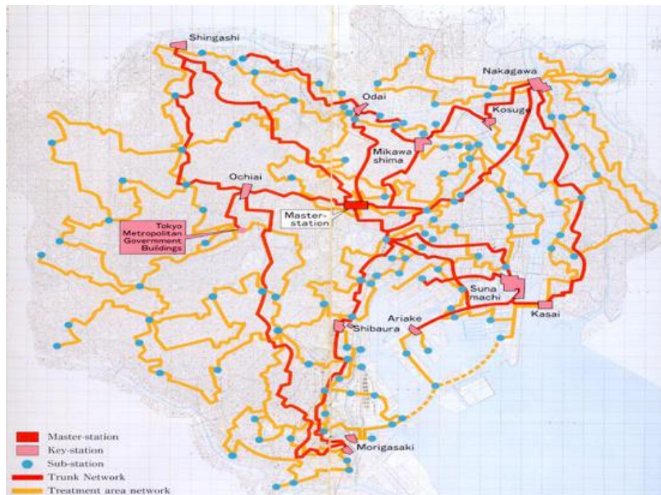
Figure 31: Fiber optic cable network in Tokyo's sewage system
