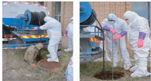
Figure 32: Conducting Sampling and Testing of Sewage Water Quality
