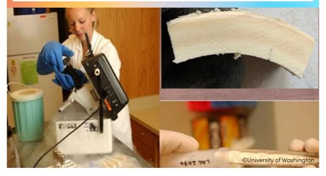
The team cuts a 3cm x 3cm sample, at least 0.5 cm thick, near the base of the tusk, where the DNA is most concentrated. The sample is put into a machine that uses liquid nitrogen to help pulverize it into a fine powder.
