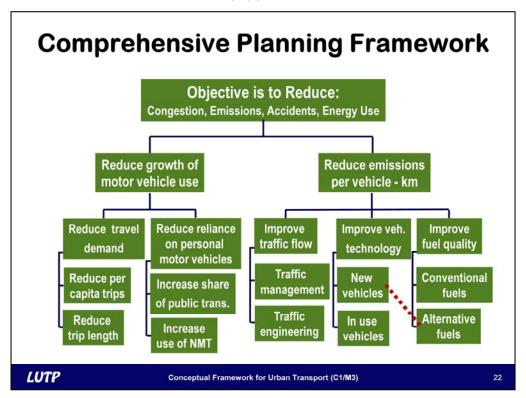
Alternative fuels will generally be possible only for new vehicles, though there have been examples of cleaner fuels being introduced in old vehicles as well, such as the use of CNG kits in diesel buses. The buses can be the same, but a CNG package can replace the diesel fuel system. In some cases this is possible.
