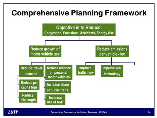
Improving vehicle technology is another way of reducing emissions per vehicle-kilometer. Vehicles that are more energy-efficient and consume less fuel per kilometer are more efficient. Many countries have established stringent emission norms to regulate emission levels.
