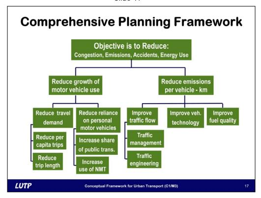
... traffic engineering. When vehicles move in the same lane, but at different speeds, the slowest vehicle determines the speed of the traffic. Segregating slow-moving vehicles from fast-moving vehicles can help improve traffic flow. Similarly having lanes for different speeds help improve traffic flow.
