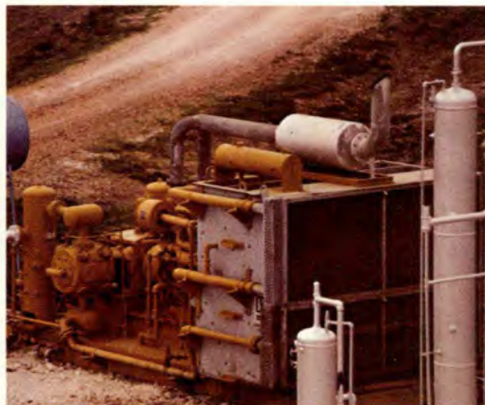
RESERVOIR DEPLETION application near Refugio, Texas employs a two-throw, five-inch (12.70 cm) stroke "FE" compressor to handle pressure of 85 psi (5.98 Kg/cm 2 ) and discharges at 950 psi (66.79 Kg/cm 2 ).
