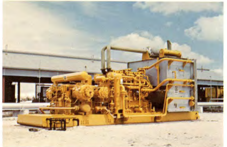
SALES GAS compressor installation in south Texas uses a five-inch (12.70 cm) stroke, four-throw "FE" compressor operating with 70 psi (4.92 Kg/cm 2 ) intake pressure and discharging at 900 psi (63.28 Kg/cm 2 ).
