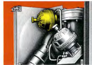
Natural Gas Manifold Pressure Regulation
