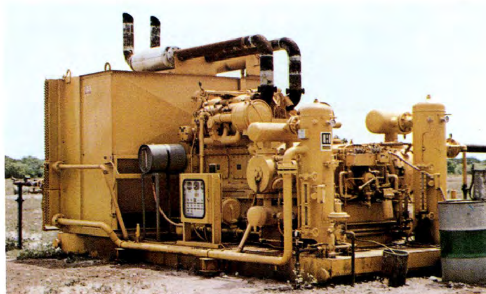
Class "FE" — balanced-opposed compressors with 5" and 6" strokes and horsepowers from 250 to 2400.
