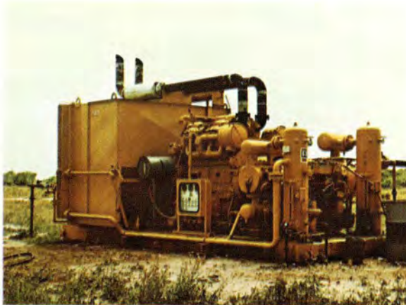
SALES GAS compressor installation in south Texas uses a five-inch (12.70 cm) stroke, four-throw "FE" compressor operating with 70 psi (4.92 Kg/cm 2 ) intake pressure and discharging at 900 psi (63.28 Kg/cm 2 ).
