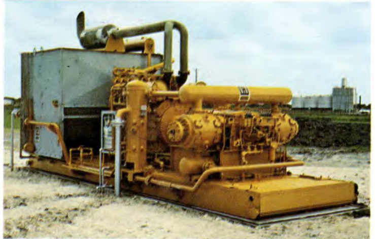
RESERVOIR DEPLETION employing a five-inch (12.70 cm) stroke, two-throw "FE" compressor near Refugio, Texas.
