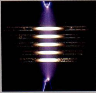
R&D work at NTT extends to production technology, as in this apparatus, which fuses joints in five optical fibers simultaneously (above).
