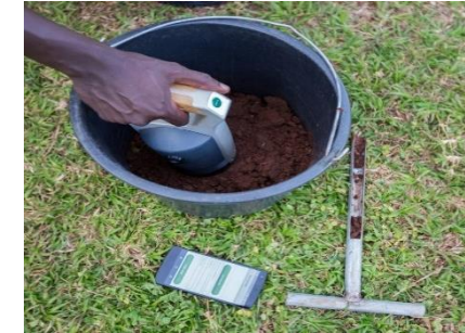
AgroCares: IoT soil scanner
