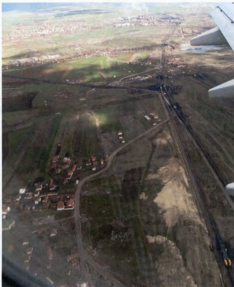
Figure 1. A Conveyor belt moves lignite from the open pit (right) to the Kosovo A power plant (top center). The community of Hade (left center) is scheduled for forced displacement. The bulldozed remains of earlier displacements are to the right of road (right, lower center). Photo T.Downing
