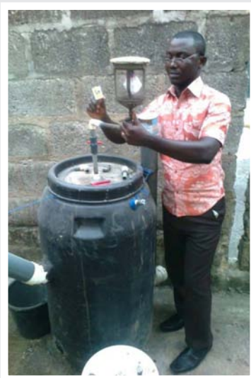
The first portable biogas plant prototype. © World Bank.
