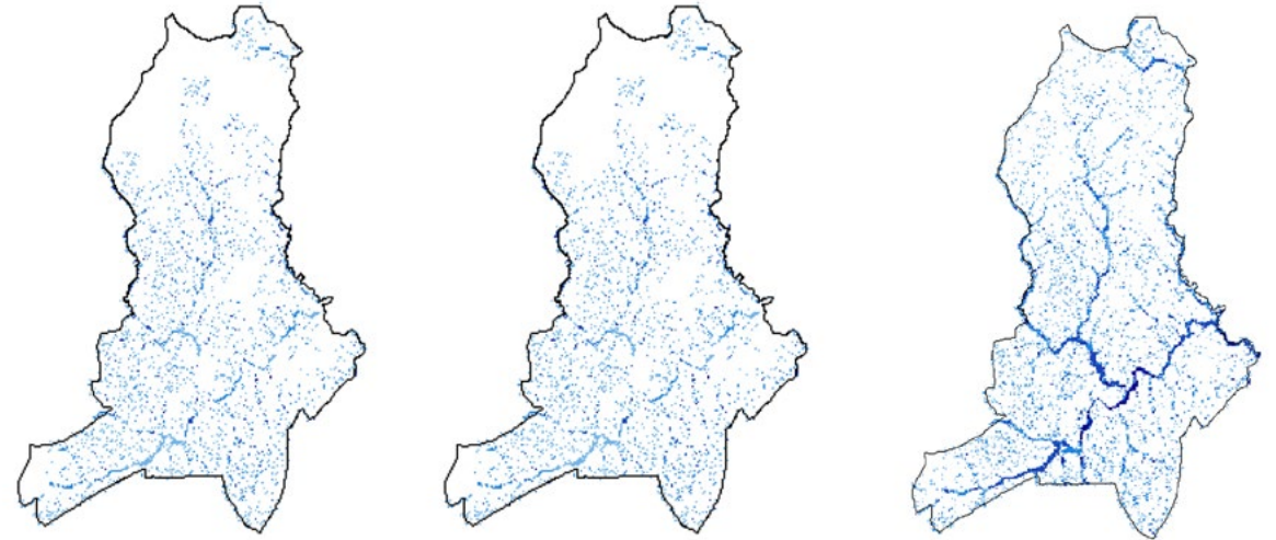
Figure 30. Flood Inundation Results for Lilongwe for 50 (left), 100 (center), and 250 mm (right) Storms
